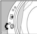
To disable this device and restore the possibility of closing the door, rotate the button anti-clockwise until the groove is vertical.
