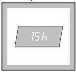
The delay time is displayed for 3 seconds, then the duration of the selected programme reappears. After you have pressed the START/PAUSE button, the countdown begins, and the delay time value decreases by one unit every hour till the first 2 hours, and then it decreases by one unit every 30 minutes.
