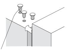
Carefully remove hole plugs from holes to allow fitment of the top bracket.
