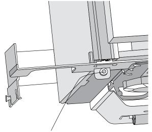
Tension on the centre cover can be adjusted with the screw on the bottom bracket
