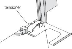
Engage the centre cover piece into the tensioner of the bottom bracket. To facilitate this loosen the tensioner if required.
