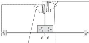
Two cabinets of different depths joined at the back with rear clamp. Notice that compressor mounting plate fasteners are in a different location on the rear clamp.
