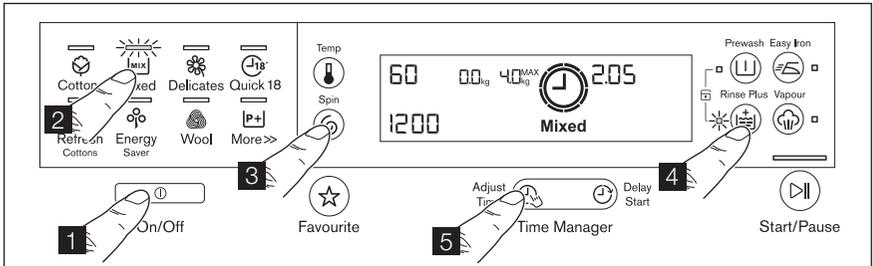
**i** For a correct operation of the weight sensor, activate the appliance and set a wash program **BEFORE** loading the laundry in the drum.
