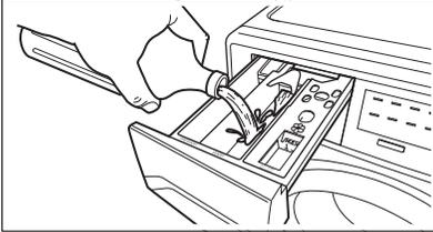
3. Select a Cottons cycle at 90 °C, without any laundry in the machine, to remove any manufacturing residue from the drum and tub. Pour 1/2 a measure of detergent into the dispenser drawer and start the machine.
