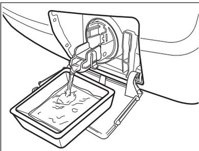
5. When the container is full of water, put the drainage duct back again and empty the container. Do steps 4 and 5 again and again until no more water flows out from the drain pump.
