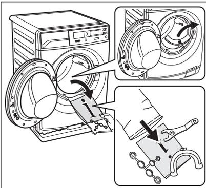
5. Open the door. Remove the polystyrene piece from the door seal and all the items from the drum.
