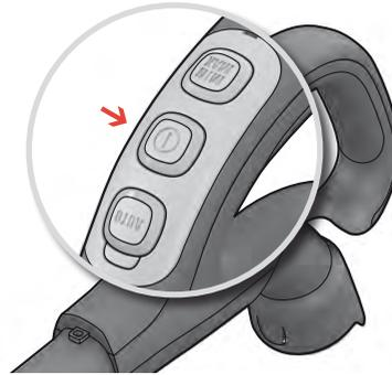
**8. Models with remote control** can also be operated by the ON/OFF button on the handle.
