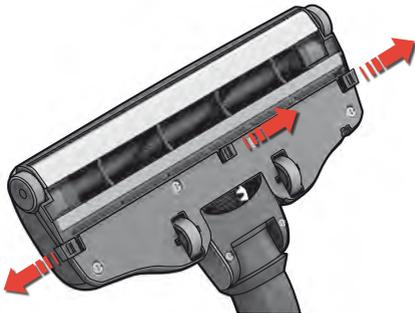
1. **Open brush roll cover by pushing the latches.** This will free the front wheels for cleaning.
