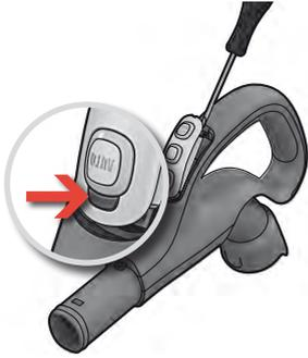
**1. Change battery when** light indicator is not responding when pressing any button.
