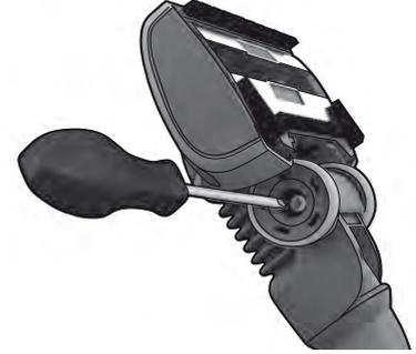
3. Unscrew the wheel axis and clean all parts. Refit in reverse order.
