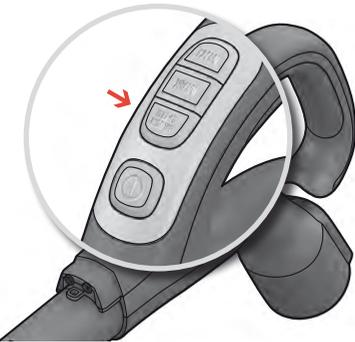
**11. Models with remote control and AeroPro motorized nozzle.** To turn the motorized nozzle on and off, press BRUSH button on the handle.
