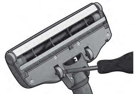
3. **If the wheels are stuck**, remove them carefully by using a small screwdriver.
