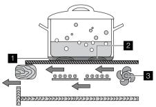
Cracking noise 1 when using cookware made of different materials (Sandwich construction)
