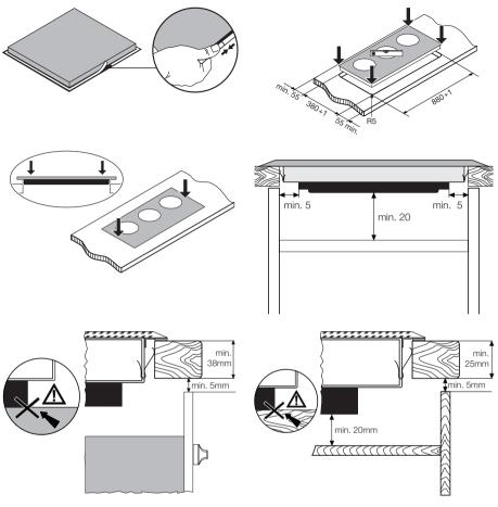
✓ Warning! Surface temperatures of base exceed 95°C, under bench access must be restricted by use of
