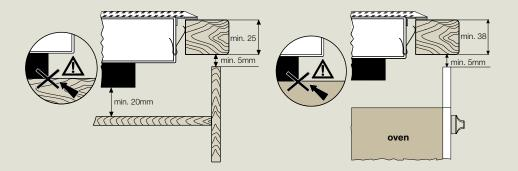
WARNING: Under no circumstances should the cooktop base be installed directly onto a shelf.
