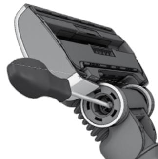
Unscrew the wheel axis and clean all parts. Refit in reverse order.
