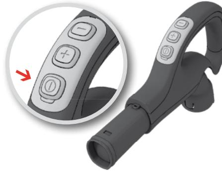
**Models with remote control** can also be operated by the (ON/OFF) Ⓛ button on the handle.
