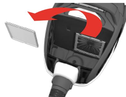
Pull the grip and remove the filter frame.
